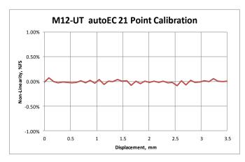
Flexibility is particularly evident in the linearity calibration options included with the *auto* EC. The charts on the left are typical output curves for the *auto* EC with the M12–UT probe.
