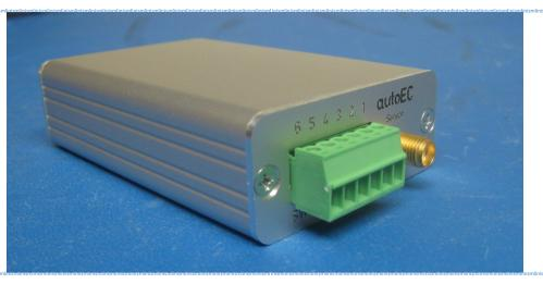
an innovative digital driver designed for *high precision, high resolution* using passive eddy current position/displacement probes
