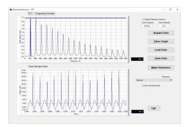
*auto* EC has the capability to collect 512 samples at the chosen sample rate, upload the data to a PC, and do an FFT on the data. This can be useful for machine monitoring and complex analysis.
