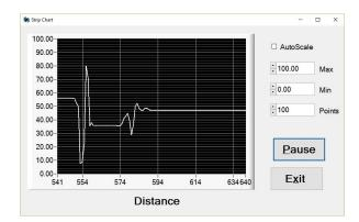
The strip chart allows graphical display of the output in real time. It can auto scale from 0-100%, or the min and max scales can be set to display whatever output is selected. If 0-10VDC is the output, simply set min to 0 and max to 10.
