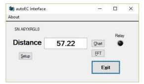
The interface screen displays the sensor output and allows access to the Setup, Calibration, Strip Chart and FFT screens.
